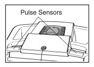
grip pulse sensors, with your hands on the metal contacts. Avoid moving your hands. After a few seconds, the PULSE indicator below the Calories/ Pulse display will light, and then your heart rate will be shown. For the most accurate heart rate reading, continue to hold the contacts for about 15 seconds.
